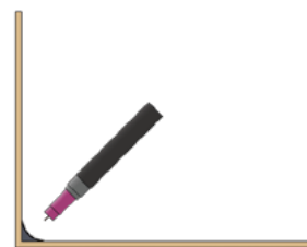
▲ Flat Corner Welding
